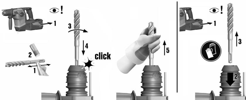
1. Lightly grease the connection end of the accessory tool.
