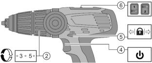
Set the forward/reverse switch to the desired direction of rotation.
