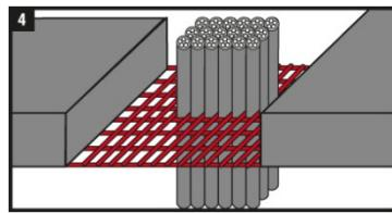
When closing floor openings, fasten wire mesh in place as shown in drawing.
