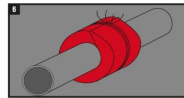
If required, wrap cable/cable tray resp. pipe with Hilti Firestop Cushion CFS-CU L and fix with wire as shown in drawing (please refer to Annex C).
