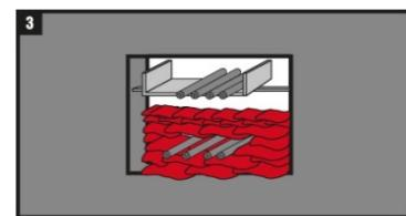
Cushion arrangement with cables/cable trays running through wall partition.
