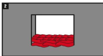
Cushion arrangement without cables running through wall partition.
