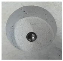
Locally exposed steel with shiny ring after PFP-removal operation
