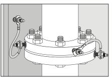
Functional and protective bonding of pipes<sup>5</sup> (outer diameter of installed surface  $\geq$  150mm)
