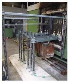
Figure 2: Test facility for fire test (small bulkhead)
