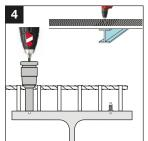
Screw-in S-BT studs into drilled hole.
