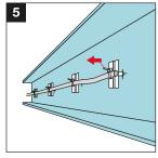
Screw-in S-BT studs into drilled hole.
