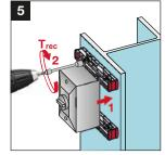
Fasten the accessory on the channel with the suited installation torque.
