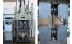
Test facility for fatigue test
