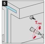
Tighten the standoff adapter with the recommended installation torque  $T_{rec}$  of 8 Nm.
