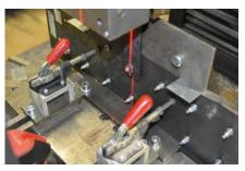
Test set up for shear load testing
