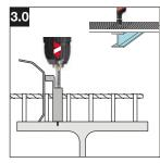
Pre-drill with TS-BT 5.5-110 S stepped drill bit and S-CS NG centering spacer.
