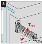
Fasten the accessory on the standoff adapter with the recommended installation torque  $T_{rec}$  of 20 Nm.
