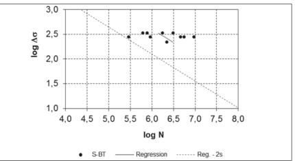
As often done in fatigue design, the characteristic resistance  $\Delta\sigma_k$  (= 5%-fractile or 95% probability of survival) is assessed by reducing the linear regression with the double of the standard deviation "s" of the test data. "s" corresponds to the standard deviation of the difference between the test results and the mean trend. Applying this procedure, the characteristic fatigue strength determines to:
