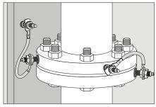
Functional and protective bonding of pipes (outer diameter of installed surface ≥ 150 mm)
