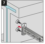
Position accessory on standoff adapter and hold in place. Use of MQZ bore plate as needed for strut applications.
