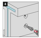
Set S-BT studs into drilled hole using the S-DG BT depth gauge.
