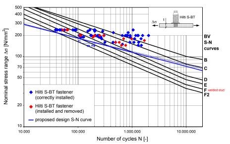
Figure 4: Comparison of Hilti S-BT fatigue test data with BV:2016 fatigue curves and new proposed fatigue curve "S-BT" for Hilti S-BT fastener
