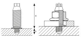
Figure 3: Geometry of S-BT studst
