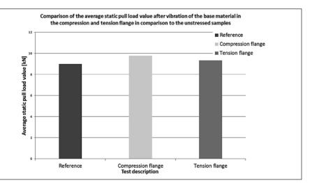
Ultimate pull-out loads of S-BT fasteners before and after cyclic loading of the steel beam
