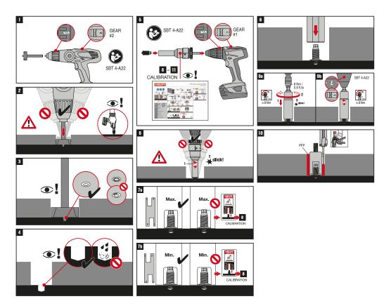
4.16.2 Instruction for use – Fastening of standoff adapter with S-BT on PFP-coated steel
