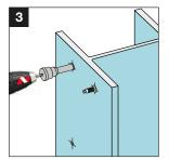
Screw-in S-BT studs into drilled hole.
