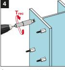
Screw-on the Hilti standoff adapter on the S-BT stud and tighten it with the suited installation torque.
