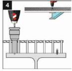
Screw-in S-BT studs into drilled hole.
