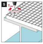
Tighten X-FCM NG discs with 5 mm Allen-type bit with the suited installation torque.
