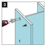
Screw-in S-BT studs into drilled hole.
