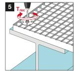
Tighten X-FCM discs with 5 mm Allen-type bit with the suited installation torque.
