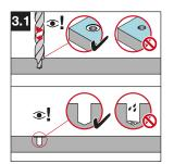
Pre-drill until shoulder grinds a shiny ring. The drilled hole and the area around drilled hole must be clean and free from liquids and debris. 2
