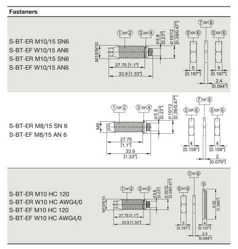
**Report No. 17-IK-0093.S02:** Suitability of Hilti S-BT-ER and S-BT-EF threaded studs as connection point in protective grounding and earthing circuits and for lighting protection; Electrosuisse, Fehraltorf, Switzerland; July 2017
