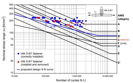
Figure 2: Comparison of Hilti S-BT fatigue test data with AWS D1.1:/D1.1M:2015 fatigue categories and new proposed fatigue stress category "S-BT" for Hilti S-BT fastener
