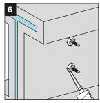
Close the opening within 4 hours of the opening is being made in accordance to the patching instructions by the PFP-manufacturer.
