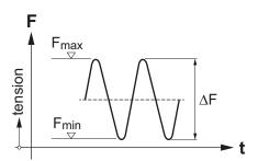
Principle sketch of cyclic tension tests
