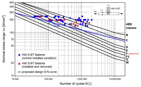
Figure 3: Comparison of Hilti S-BT fatigue test data with ABS-(A) Offshore S-N curves and new proposed fatigue class "S-BT" for Hilti S-BT fastener
