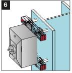
Fasten the accessory on the channel with the suited installation torque.
