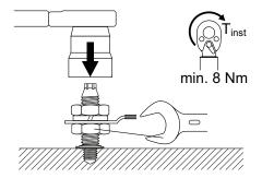
Single point connection type A and double point connection type A
