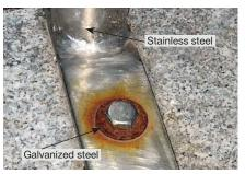
This is a typical case of contact corrosion. Zinc-plated carbon steel (washer) and stainless steel (screw and part) were used together. The surface area of the more noble metal – the stainless steel – is larger, causing strong corrosion of the washer.
