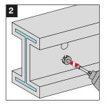
Remove PFP and pre-drill with TS-BT 31-74 PFP stepped drill bit...
