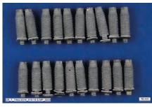
Removed S-BT fasteners after 12 weeks EN ISO 16701 cyclic corrosion test. No visible corrosion.
