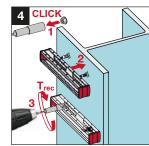
Position channel on S-BT studs and hold in place. Tighten the nuts with the suited installation torque.
