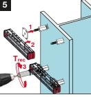
Position channel on standoff adapter and hold in place. Tighten the nuts with a tightening torque  $T_{rec}$  of 20 Nm.
