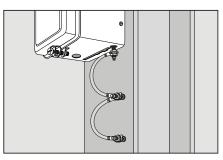
Protective bonding circuit – Double point connection
