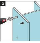
Screw-in S-BT studs into drilled hole.
