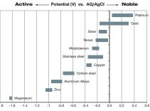
Corrosion potential of various metals in sea water
