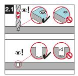
Pre-drill until shoulder grinds a shiny ring. The drilled hole and the area around drilled hole must be clean and free from liquids and debris.
