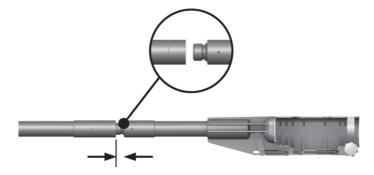
Screw the tubular sections and tool holder together, tightening the joints by hand only, without use of tools.
