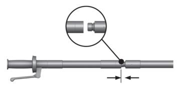
Screw the tubular sections and grip section together.
