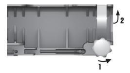
Open the retaining bar by releasing the screw knob.
