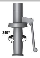
The grip section can be rotated at any time to bring it into a comfortable working position.
