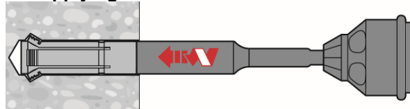
6. Applying hammer drill
